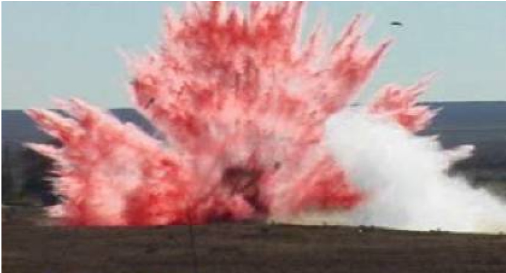
Fig. 1. Dispersed water (dyed red) at furthest extent radially from impact (Jepsen et al., 2004). Frame is approximately 92 m wide and was acquired 2 s after impact.
